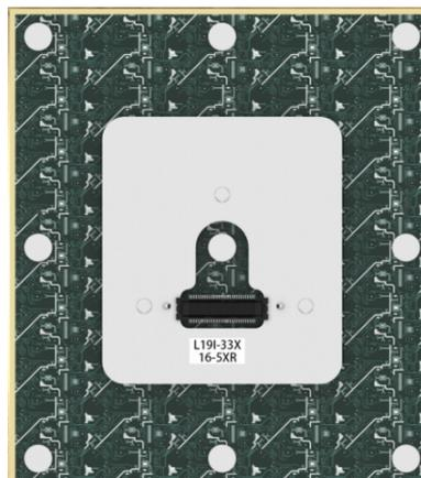
3. To achieve a better display effect, you can install the modules according to their serial numbers at the time of factory correction, as indicated in the diagram.
