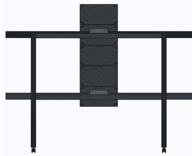
3. Install the panels in the rest of the columns, as illustrated below:
