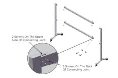
④ Tighten the mounting screws with the appropriate tools and the brackets are assembled, as shown below:
