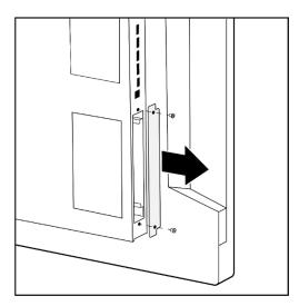
II. Install the Avocor OPS computer by carefully sliding it into the OPS slot as pictured below.
