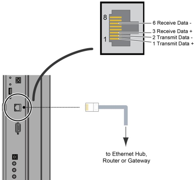
Figure 3-3. Ethernet Connection
