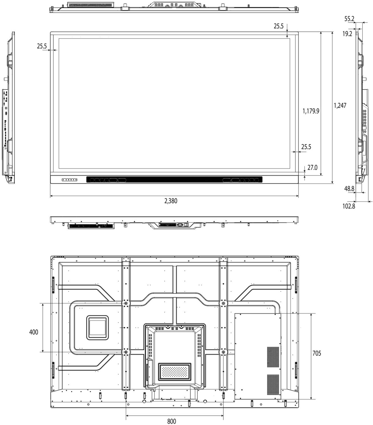
**Figure 7-2. AVF-8650 Display Dimensions (mm)**
