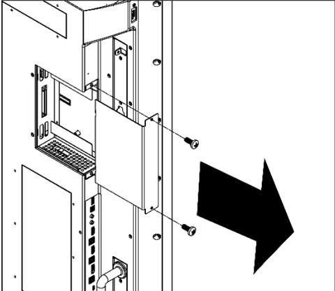
VI. Install the OPS computer by carefully sliding it into the OPS slot as pictured below.
