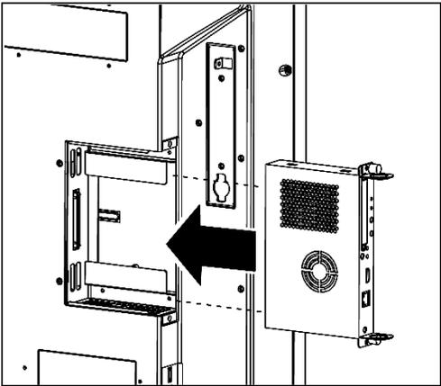
VII. Secure the OPS computer into the slot using the screws that were removed earlier
