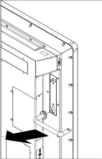
V. Remove the OPS slot shield on the display input panel
