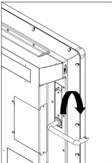
IV. Take off the handle carefully on the display input panel
